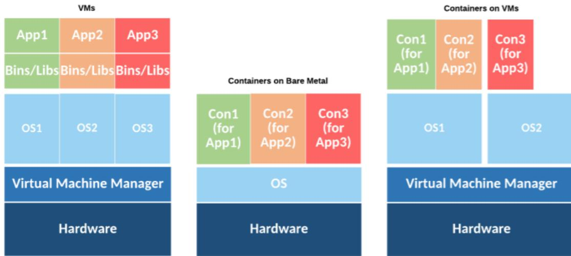
Figure 2: Virtual Machine and Container Deployments
